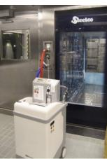
As an alternative to the  $H_2O_2$  vapor generator the AC 7500 can be connected to a chlorine dioxide generator.
