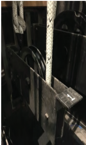
Picture above shows tension block installed upside down. True for all Tension Blocks in the system
