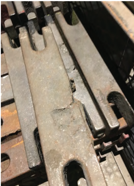
The images above show Cast counterweights. The weights are noticeably deformed.
