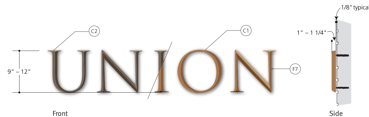
2 Detail ST33C scale: 1"=1'-0"
