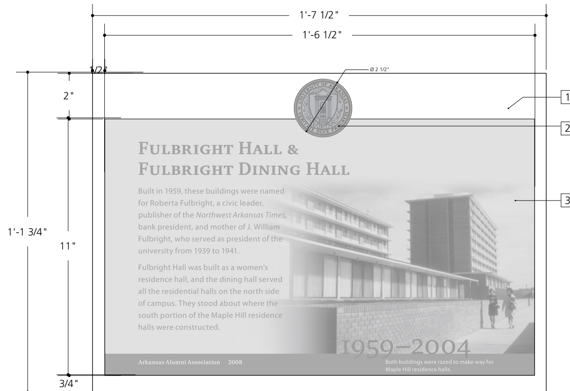
1 Flat Elevation of Interpretive Panel scale: 1 1/2"=1'-0"
