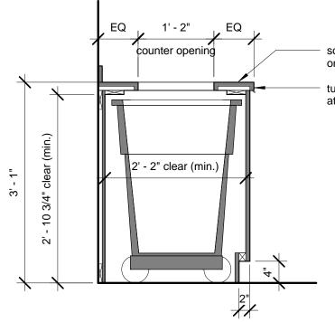
solid surface counter on plywood substrate
